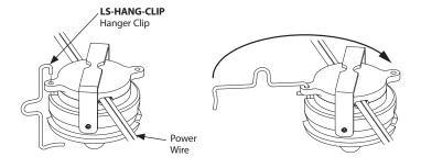
**Step 6:** Position first socket below suspension cable and swing hanger over the cable and across the top of the Litesphere<sup>™</sup> socket and the Shade Adapter Bracket.
