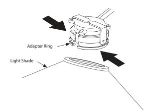
**Step 2:** Hang the lip of the Shade opening over the lip of the Adapter Ring at the point where the Adapter Ring is pressed together.
