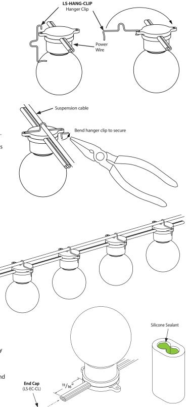
**Step 3:** Position first socket below suspension cable and swing hanger over the cable and across the top of the Litesphere<sup>™</sup> socket.
